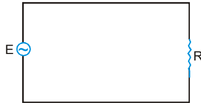
AC voltage applied to a resistor
